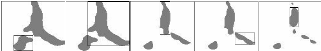
(a) The found blobs from analysis of a 2-D histogram of horizontal motion and binocular depth disparities. In the sliced histogram shown, motion is in the horizontal direction and relative depth in the vertical direction. The bounding box blob approximation that we use is circumfering the peaks in the histogram. Shown in grey is the histogram slice at the start level of each blob.
