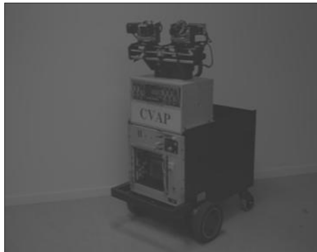
Figure 1.2: The head-eye platform used for the experiments in (Nordlund and Uhlin, 1996).
