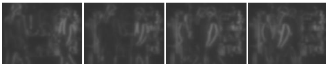
(c) Certainty maps computed corresponding to the disparity map. The lighter, the higher certainty.
