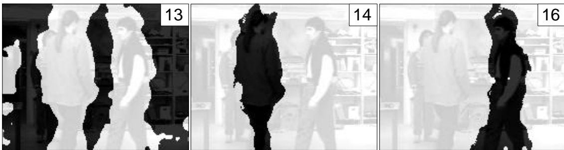
Figure 1.8: Example of backprojected blobs (marked with darker colour). Number in upper right corner refers to blob-number in Figure 1.7.
