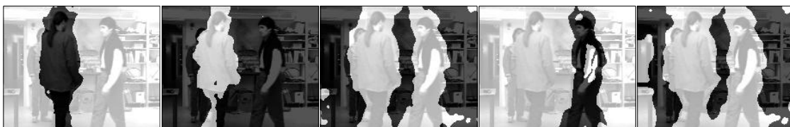
(d) The final backprojection. The backprojections shown in Figures 5.2(b) and 5.2(c) combined with logical AND.
