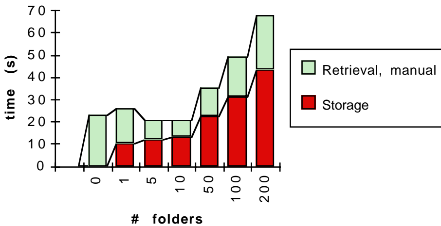
Figure 6.8 Time for storage compared to retrieval. Manual retrieval. 500 stored messages. 4 messages to archive and 2 to search.
