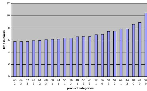
Figure 9. MTBF in the mailroom for different product categories in company one. The code 44 0 indicates a product with 44 pages and no inserts.
