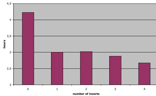
Figure 8. The MTBF in relation with the number of inserts. The value for one insert includes all different page counts in the main newspaper at company G.
