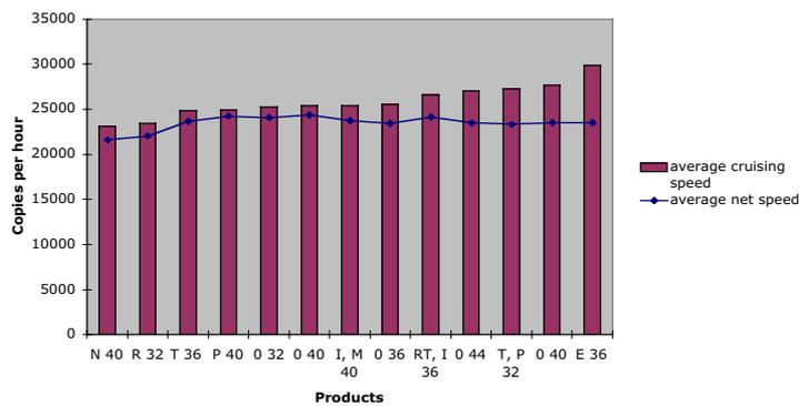
Figure 14. The average net production speed and the average cruising speed in the mailroom
