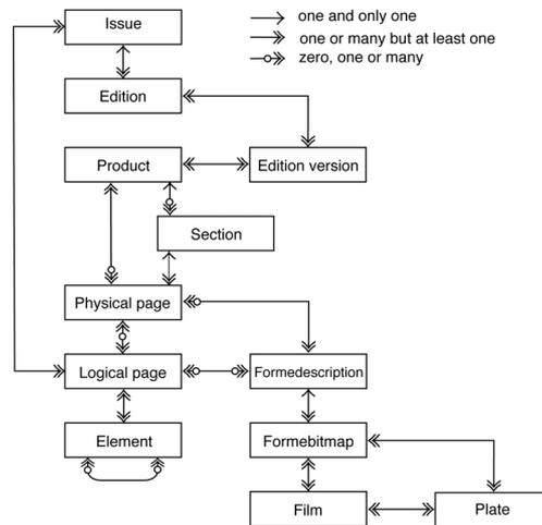
Figure 1. The IFRATRACK model of a newspaper (based on Thoyer 1995).
