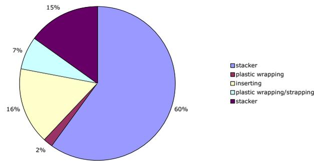
Figure 12. The minor stops divided into stop categories
