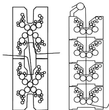
(1) The printing presses – the figures show both 4-high and satellite presses. Here the newspapers are printed. Four-high units can be arranged in different ways. As the figure shows or the four units can be arranged in the inverted way or unit two and four can be arranged inverted to form two H-type units.
